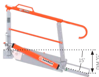
ELEVATION VIEW WORKING LOW RANGE
